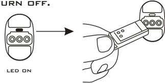
C) AFTER 4 SECONDS THE LED WILL START TO FLASH, COUNT THE FLASHES, WHEN IT STOPS FLASHING WRITE THE NUMBER DOWN ON A PIECE OF PAPER.
