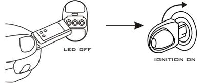
B) THE LED WILL BE ON, PLACE THE KEY INTO THE TOUCH HEAD, THE LED WILL THEN TURN OFF.
