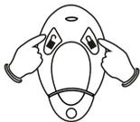
Press both buttons together when setting the alarm. The siren will sound 4 chirps and the indicators will flash twice. The sensor has now been disabled. After 20 seconds the system will be fully armed, however the sensor will be disabled.
