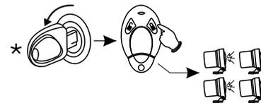
Countdown period is 90 sec. If ignition is turned off during this time, the timer will stop. When the ignition is turned on again the timer will continue. If you try to set or reset the alarm during the countdown period, the unit will sound 4 loud chirps to warn you that you are in hi-jack mode.
